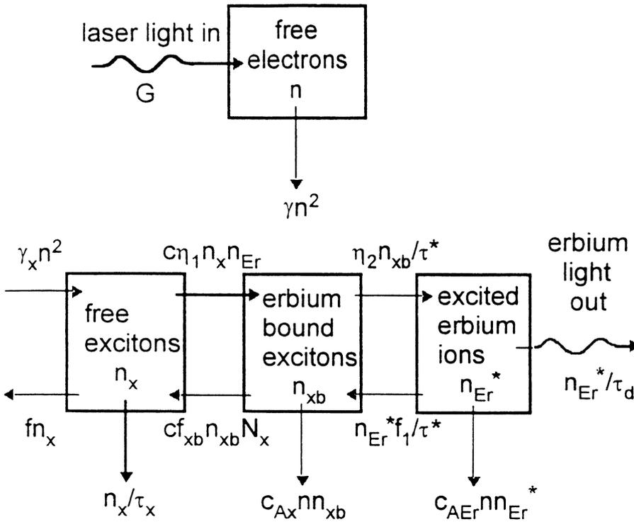
FIG. 1. Two-stream model for the photoexcitation of erbium luminescence showing generation and loss of free electrons  $n$ , free excitons  $n_x$ , erbium-bound excitons  $n_{xb}$ , and erbium ions in the excited state  $n_{Er}^*$ . Notation:  $\eta_1 = (n_{Er} - n_{xb})/n_{Er}$ ,  $\eta_2 = (n_{Er} - n_{Er}^*)/n_{Er}$ .
