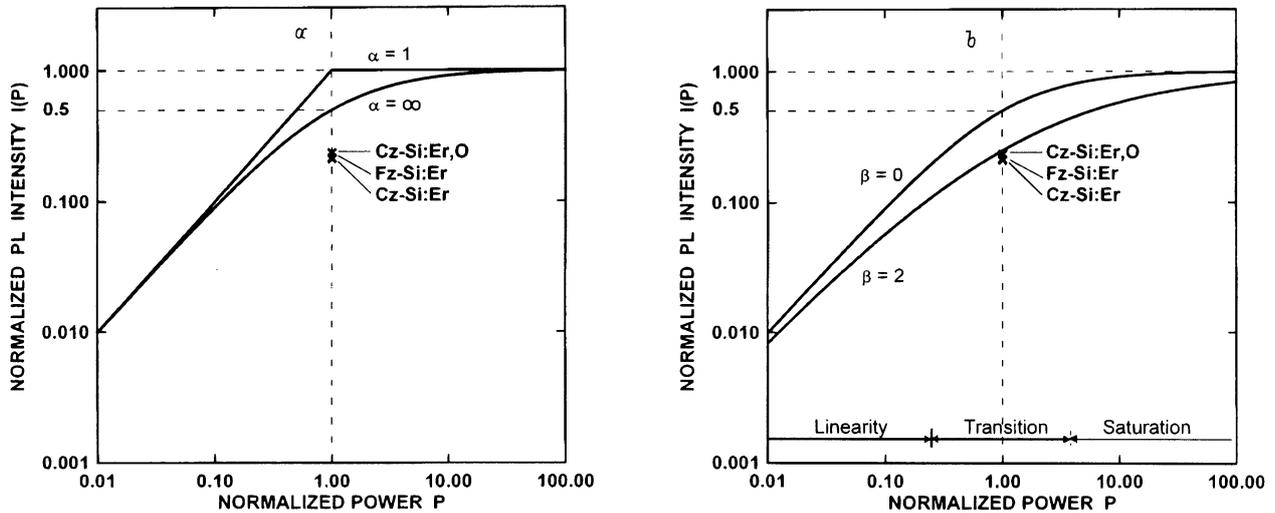
**Figure 2.** Dependence of normalized luminescence output  $I$  as a function of normalized laser power input  $P$ ; a) for the model without Auger processes, b) for a model including strong Auger decay processes. Experimental data for three samples of type  $Fz-Si:Er$ ,  $Cz-Si:Er$  and  $Cz-Si:Er,O$  are given for unit power  $P = 1$ .
