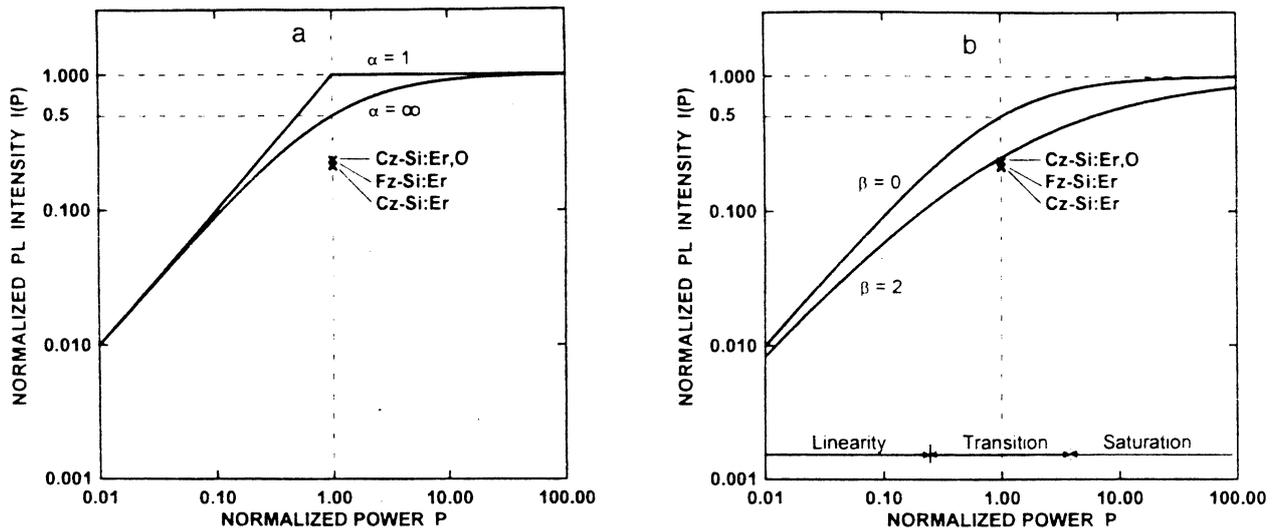
FIG. 2. Normalized luminescence output  $I$  plotted as a function of normalized laser power  $P$ ; a) for a model without Auger processes, b) for a model including strong Auger decay processes. Experimental data for three samples of type  $Fz$ -Si:Er,  $Cz$ -Si:Er, and  $Cz$ -Si:Er,O are given for unit power  $P = 1$ .
