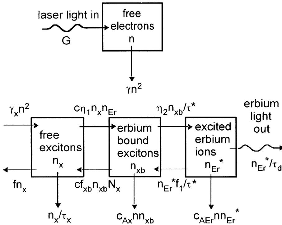
**Figure 1.** Two stream-model for the photo-excitation of erbium luminescence showing generation and loss of free electrons  $n$ , free excitons  $n_x$ , erbium-bound excitons  $n_{xb}$  and erbium ions in excited state  $n_{Er}^*$ . Notation:  $\eta_1 = (n_{Er} - n_{xb})/n_{Er}$ ,  $\eta_2 = (n_{Er} - n_{Er}^*)/n_{Er}$ .
